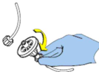
9. Repeat step 8 to connect the other end of the fluid filter.
