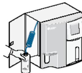
2. Remove pickup tube from Rinse container:
